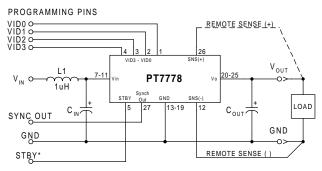
$\begin{array}{ll} C_{in} &= Required\ 2400\mu F\ electrolytic \\ C_{out} &= Required\ 330\mu F\ electrolytic \\ L1 &= Optional\ 1\mu H\ input\ choke \end{array}$
